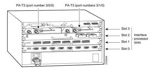
Figure 8-3 Serial Port Number Example—Cisco 7505 Shown
